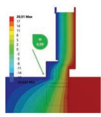
(system reduces the heat loss 4 times compared to traditional assembly)
